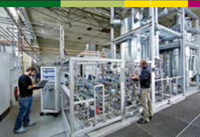
ZSW's power-to-gas plant transforms green electricity into quality gas with a methane content of 99%.
