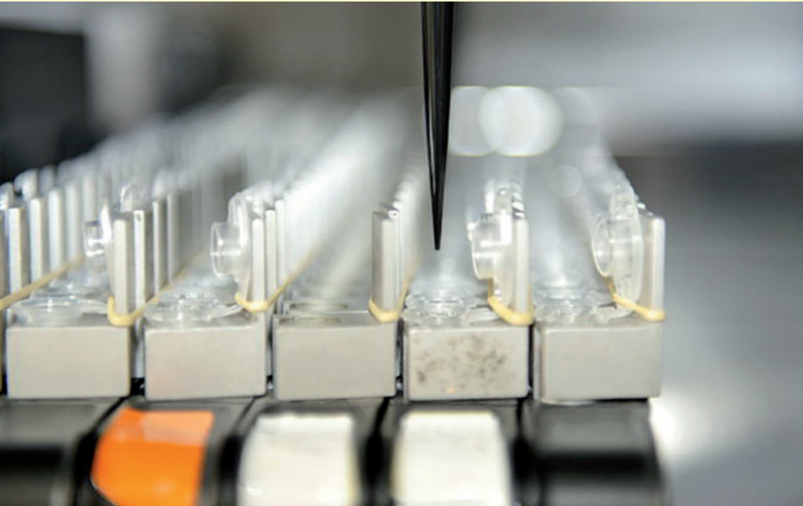
Pipetting robot for automated sample handling at GATC Biotech AG.
