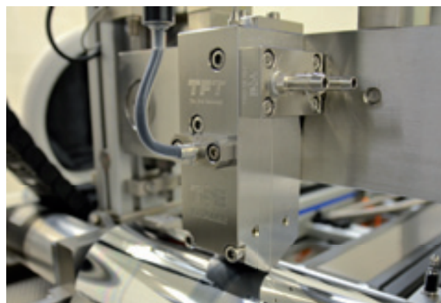
Slot die coating on high-precision slot die system.
