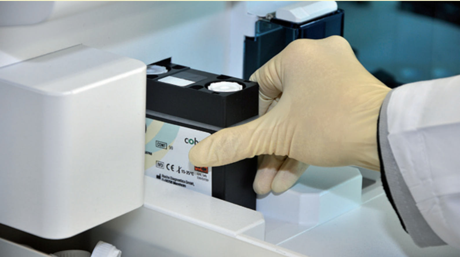
Typical reagent cartridge for current in-vitro diagnostic laboratory systems.
