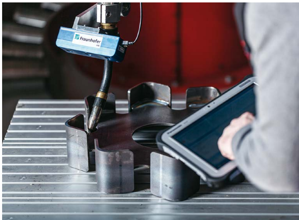
The "CoWeldRob" welding robot assistant guarantees consistent high quality welding results by automatic programme generation and process control.
