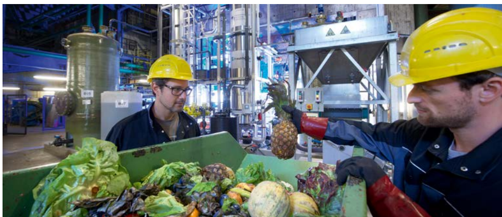
In this two-stage demonstration plant, warehouse biowaste—fruit and vegetables—is used to generate biogas. After purification, biomethane is used as a fuel for vehicles operated by compressed natural gas.
