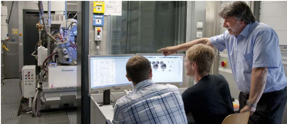
Drive-train test stand of Project Group New Drive Systems (NAS)
