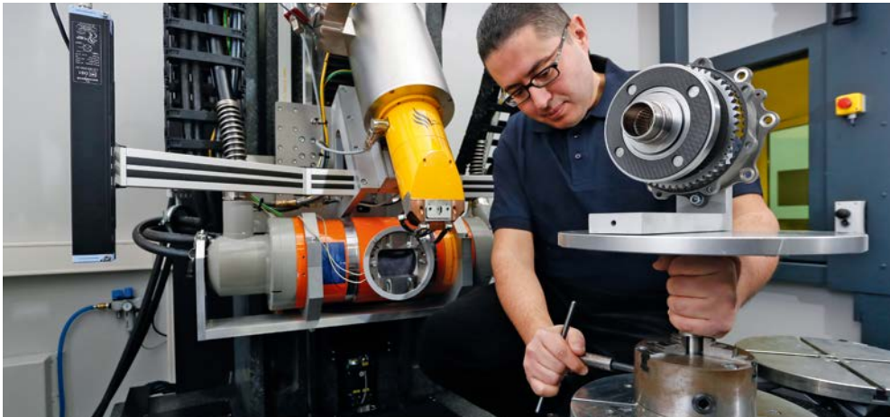
Preparations for testing a new type of propeller brake made of heavy-duty ceramic in a computer tomograph.
