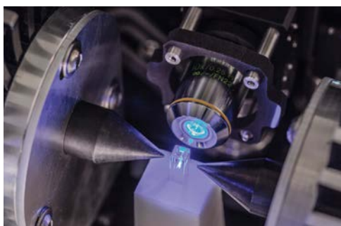
Raised signal-to-noise-ratio by concentrating the magnetic beads on a laser spot using oscillating magnetic fields.
